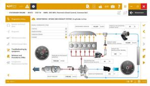
**EMR5 EDC MD1** (on SAE J1939) engine control system, System Display, activations, system checks and maintenance service operations.
